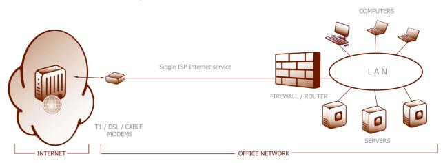
In this scenario, an SMB uses a T1 access line for Internet access. The T1 line may be used for both data access as well as for providing voice communications through a Private Branch Exchange (PBX) system. Because of this, only a fraction of the bandwidth available from the T1 line may be available for Internet traffic. Considering in addition the volume of traffic that may be consumed by incoming spam e-mail, this often leaves little capacity available for useful Internet communications.
